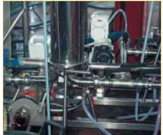
Pump on filtering pallet (wine production)
