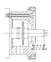
CAUTION! When mounting the new seal, plunge the parts and seals in soapy water to facilitate sliding of both the stationary and the rotary parts.
