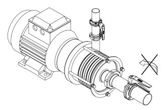
To reduce flow and motor consumption:
