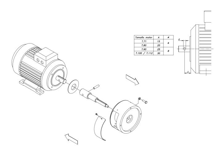
CAUTION! When mounting the new seal, plunge the parts and seals in soapy water to facilitate sliding of both the stationary and the rotary parts.
